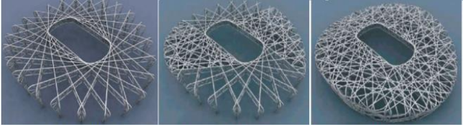
Figure 2: A model of Bird's nest stadium by M/s Arup showing the primary load carrying elements and the secondary and tertiary members (Source: Brodtkin, 2008)
